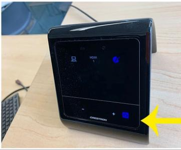
Press the power button in the lower right hand corner of the panel to power up the system. Allow for the system to warm up.
